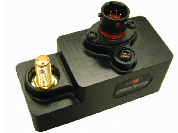
The tyre pressure receiver unit is for use with MESL tyre pressure sensors. The sensors transmit pressure, temperature, battery voltage, serial number and life count data over an RF link to an antenna on the car. Signals from the antenna are passed to the tyre pressure receiver unit where they are decoded and sent to the ECU via CAN to be further processed and scaled.
